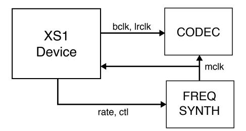
The xCORE device provides control to the frequency synthesizer and the frequency synthesizer provides the audio master clock to the CODEC and xCORE device. The sample bit and word clocks are then provided to the CODEC by the xCORE device.
